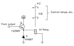
Once connected to the relay, the URC1 can turn a number of devices on and off, such as home security systems, lights, answering machine, lawn watering system, swimming pool filters, etc. Be sure the coil on the relay has a resistance of no less than 100 ohms to be safe. If it is less, use a transistor with a higher power dissipation rating.
